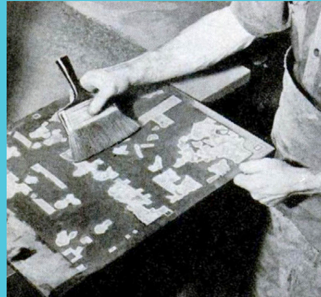
Above: Examining a zinc plate removed from the etching bath.
